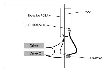
Figure 6-2 TLS-42xx Cabling Diagram
